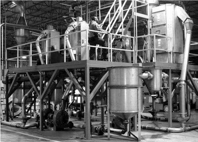
**Butler-MacDonald's system for separating plastics by using inherent specific gravity.**
