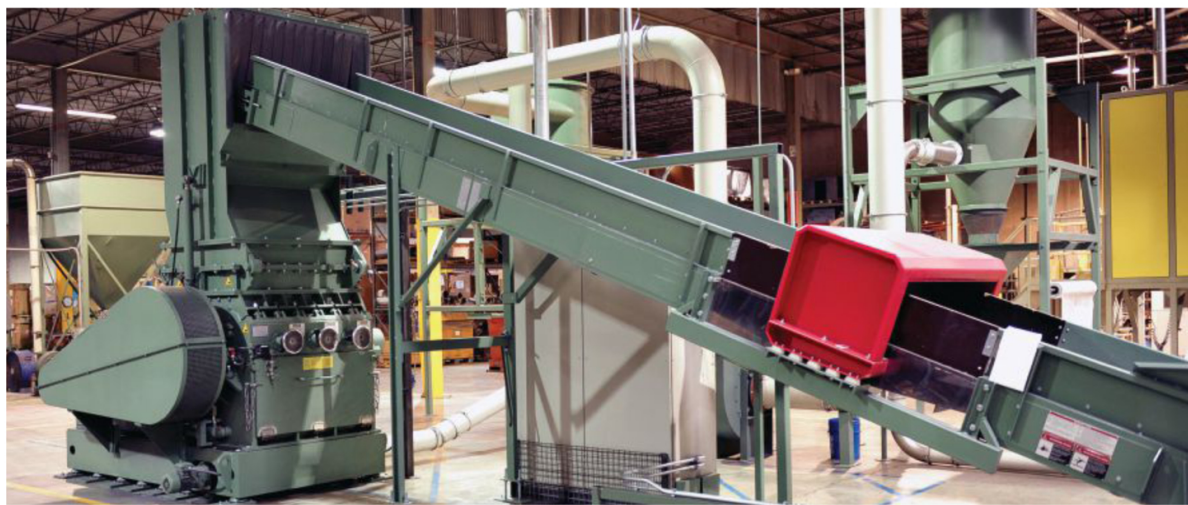
Herbold's SMS 80/120 granulator is equipped with a metal-detecting feed conveyor.
